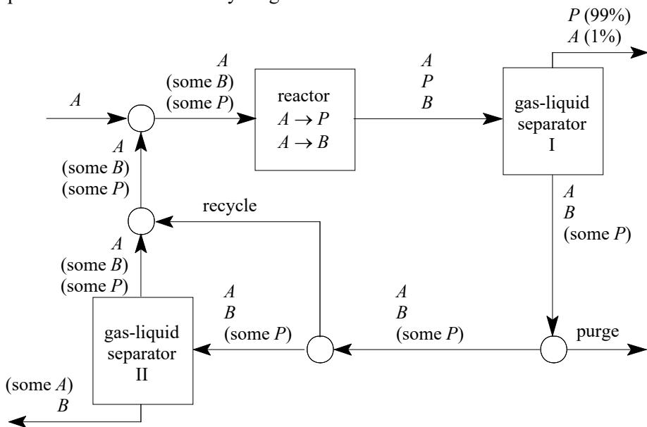
There are two options for the reactor. Reactor Type 1 has a high conversion of  $A$  but has poor selectivity for  $P$  over  $B$ . Reactor Type 2 has a lower conversion of  $A$ , but has better selectivity for  $P$  over  $B$ .
