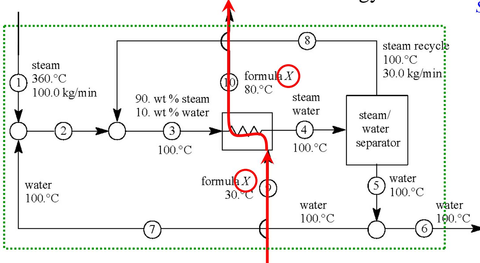
$$F_{T,9} = \frac{F_{T,1}(\bar{C}_{P,steam}(100 - T_1) - \Delta \bar{H}_{vap})}{-\bar{C}_{P,X \text{ liquid}}(T_{10} - T_9)}$$
