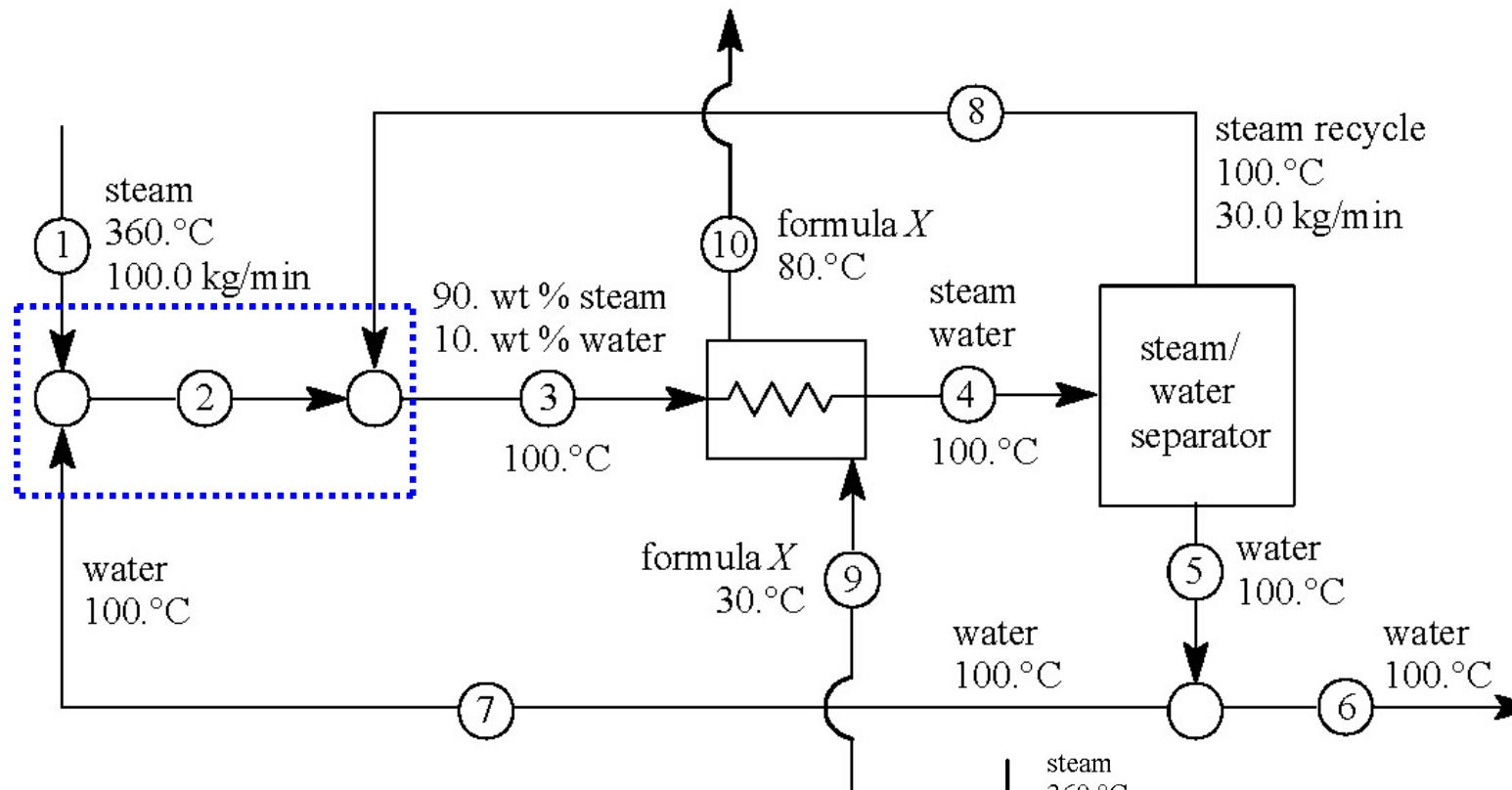
No steam in stream 8 condenses when mixed with stream 2.
