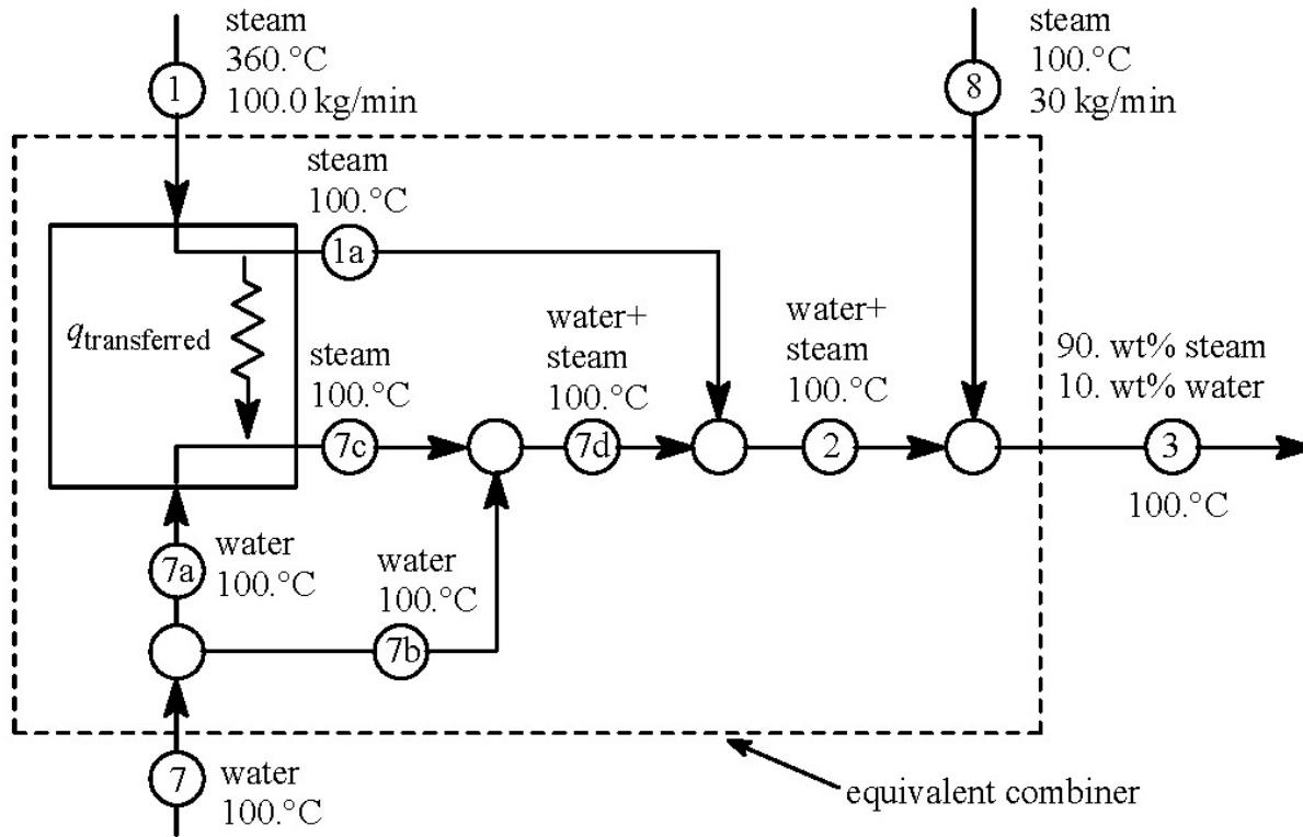
$$q_{\text{transferred}} = \Delta q_{1 \rightarrow 1a} = F_{T,1} C_{P,\text{steam}} (T_1 - 100) = 50,560 \text{ kJ/min}$$
