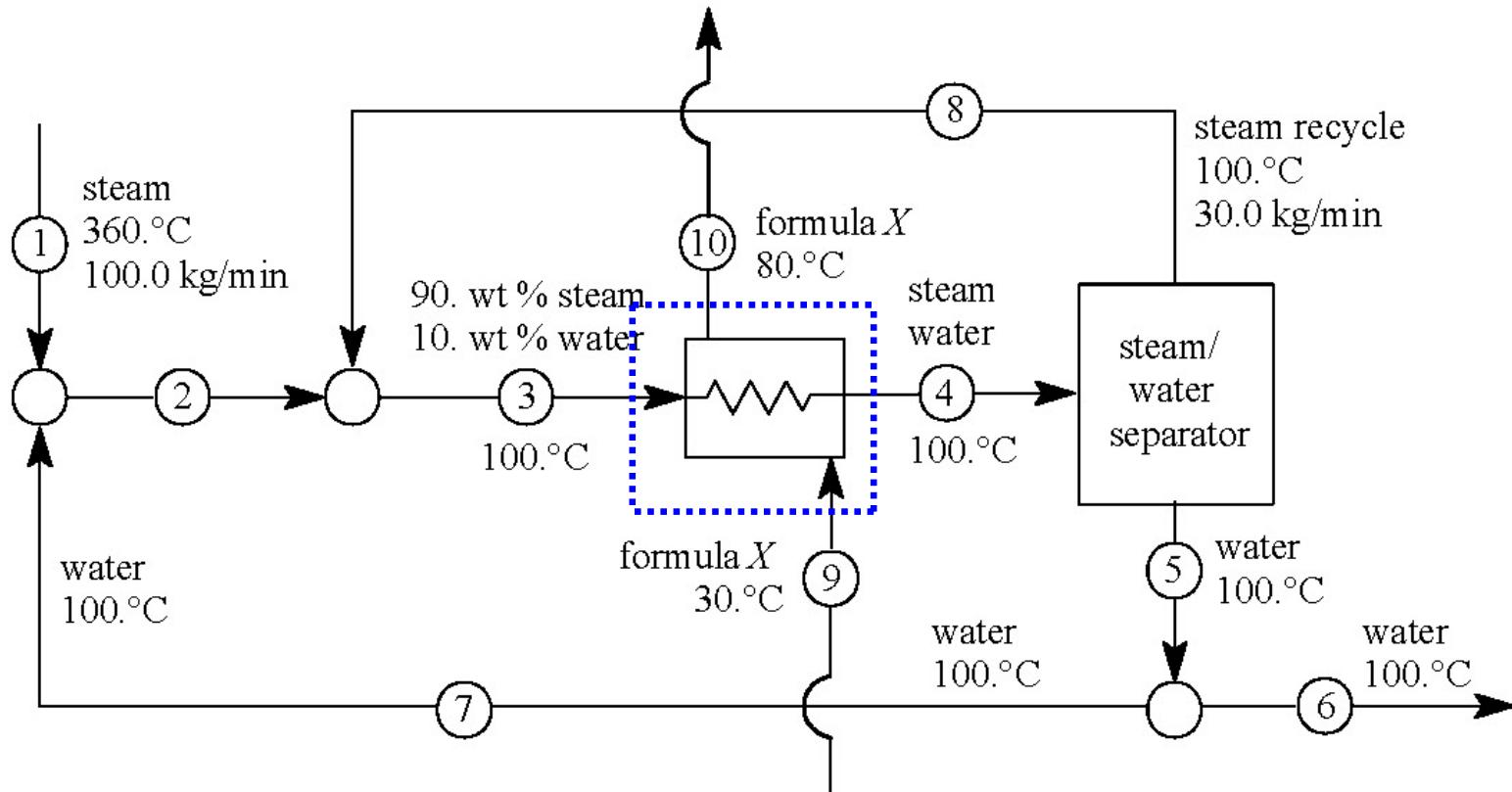
Water in stream 4 = 139.1 kg water/min.
