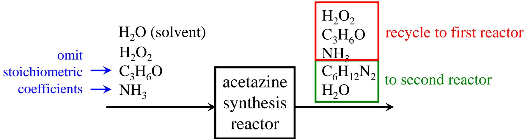
5 substances in reactor effluent. Separate into 5 streams?
