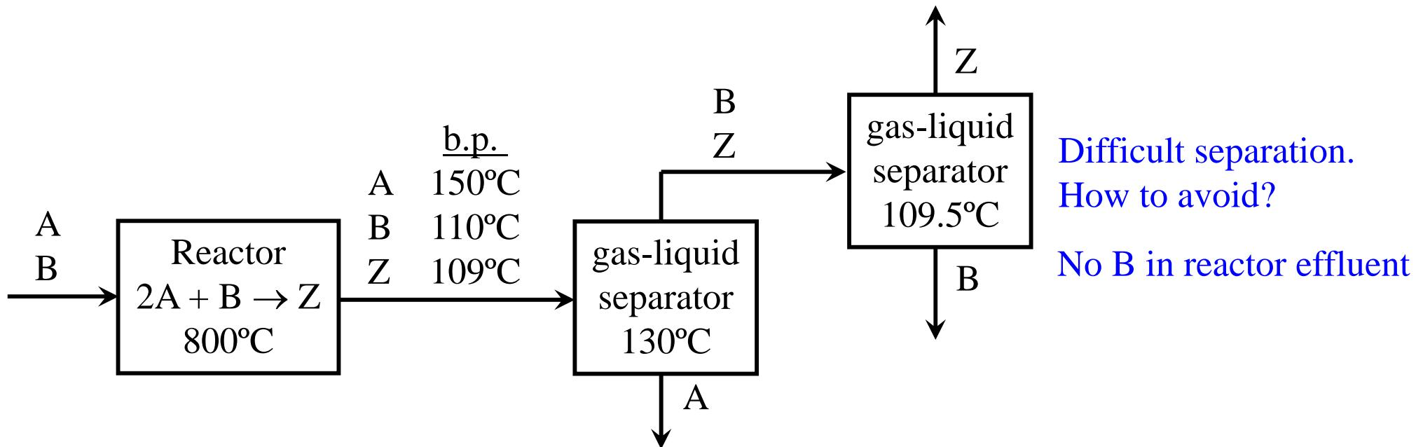
Strategy: Use excess reactant A to deplete co-reactant B in reactor effluent.
