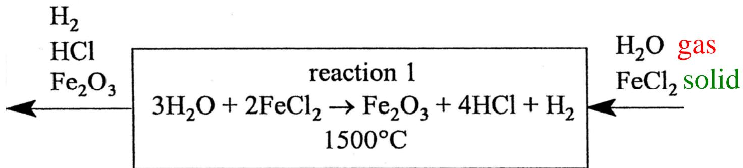
Problem: Devise a means to transport a mixture of solids and gases into, through, and out of a reactor.
