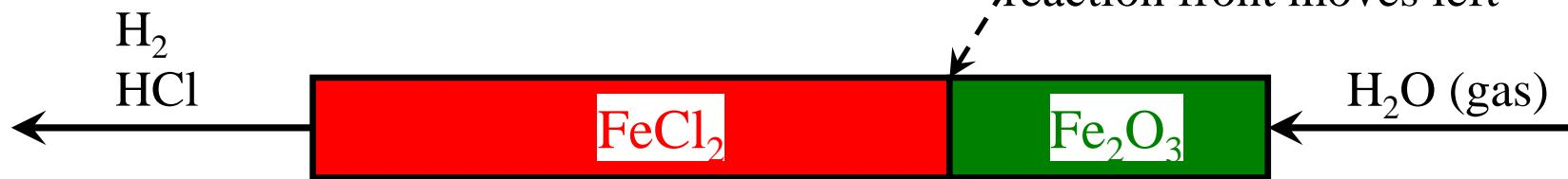
Eventually reactant gases are detected in the reactor effluent.
