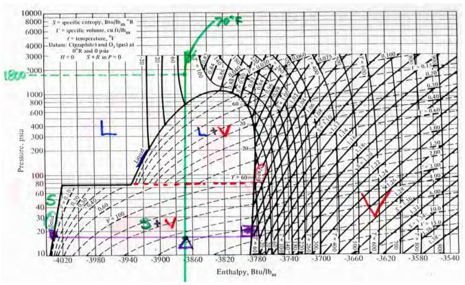
In summary, the discharge from a typical  $CO_2$  fire extinguisher is at 195 K (-108 F) and about 36% of the discharge is dry ice.
