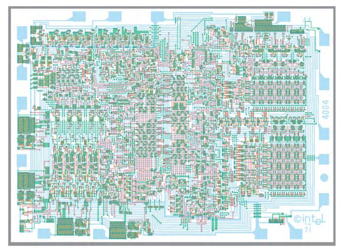
Intel's 4004 Integrated Circuit - the first microprocessor (1971) 2300 solid state transistors! Compare to 2300 electron tubes.
