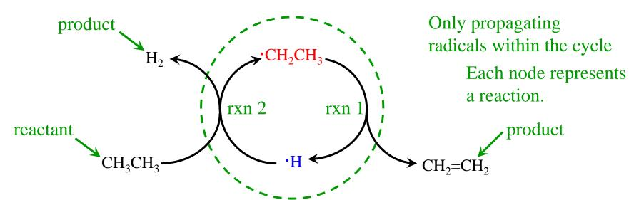
Overall mass balance consistent with overall reaction: only reactants in, only products out.
