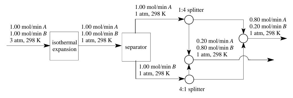
$$\Delta S_{\text{expansion}} = nR \ln \frac{V_2}{V_1} = nR \ln \frac{P_1}{P_2} = (2 \text{ mol/min})(8.314 \text{ J/K} \cdot \text{mol}) \ln \frac{3 \text{ atm}}{1 \text{ atm}}$$
